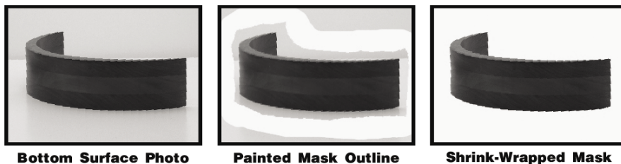
Figure 8.1.7. Masking a bottom view photo that does not include a calibration mat.
