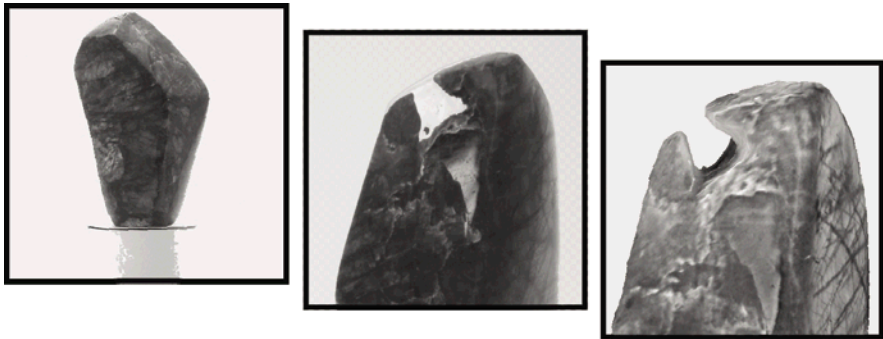
Figure 5.3.3. Mask Examples - Left mask with unmasked pedestal is OK, Center mask is overmasked causing deformity in model shown at right.
